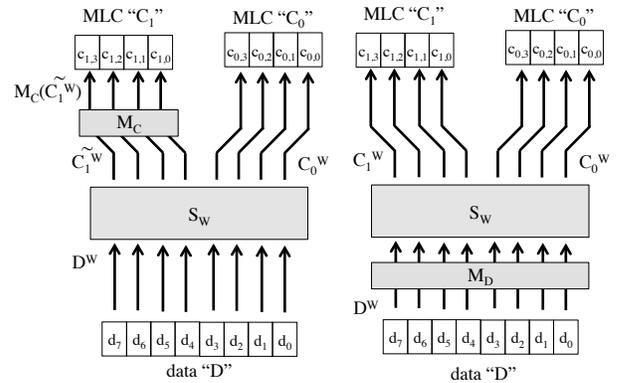
**Figure 4.** Synthesized write operations with remapping. At left is the synthesized version where the remapping is applied on the cell inputs, and at right is the final version where remapping is applied to the data word before splitting.
