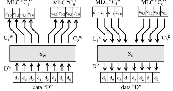
**Figure 1.** Mapping for write and read operations. At left is a write operation, where a data word  $D^W$  is distributed across two MLCs according to mapping  $S_W$ . At right is a read operation where, according to mapping  $S_R$ , data word  $D^R$  is reconstructed from the values read from the two MLCs.
