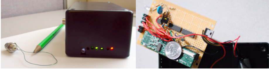
Fig. 1. Our assembled credit card emulator
